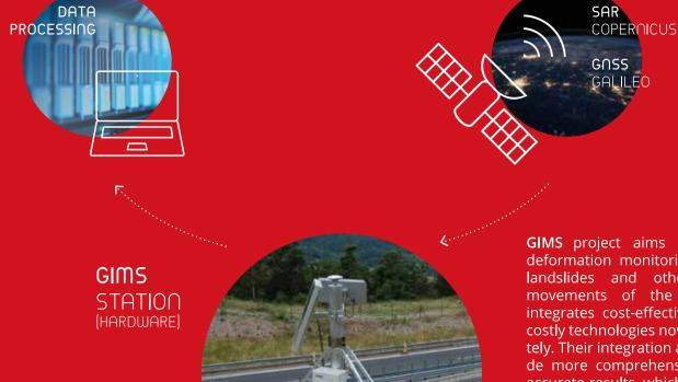
GIMS project aims at creating a deformation monitoring system for landslides and other hazardous movements of the ground that integrates cost-effective versions of costly technologies now used separately. Their integration allows to provide more comprehensive and more accurate results, which are an aggregation of images, movements and alarms.
