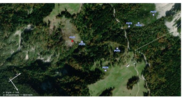
In the course of the project, fourteen GNSS stations have been installed in the **Vipava** and **Potoska** areas in Slovenia, on landslides and on a viaduct affected by them.
