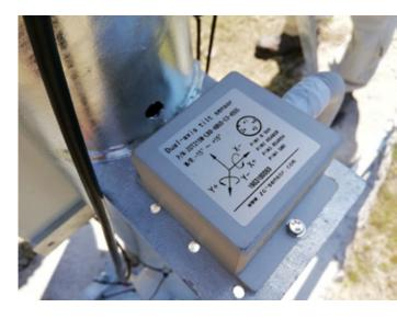
The procedure followed to process the GIMS inclinometer raw data firstly relies on a **high frequency filter** of the recorded signal and then a decorrelation from temperature.
